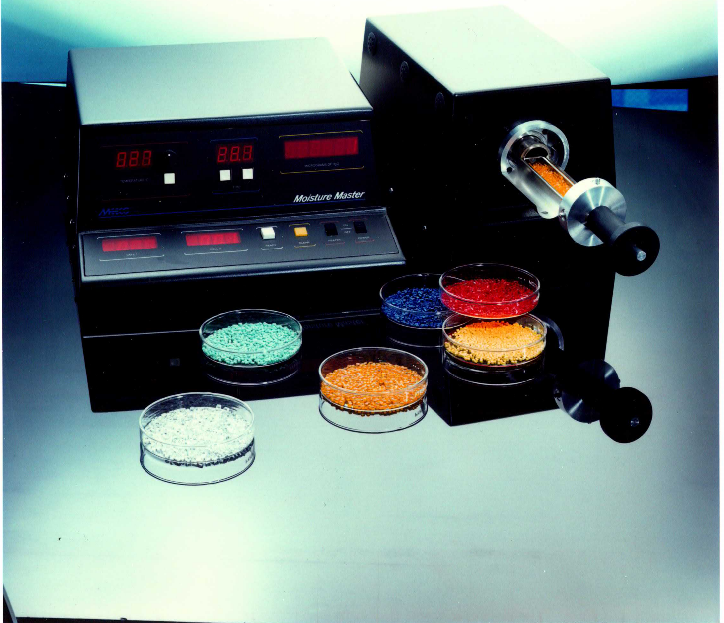
MEECO Moisture Master used to analyze moisture in solids.
